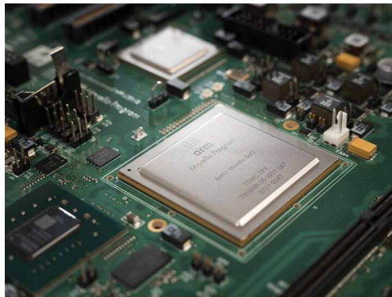
Figure 1: The Arm Morello SoC on TSMC 7FF process technology on the Morello prototype board
