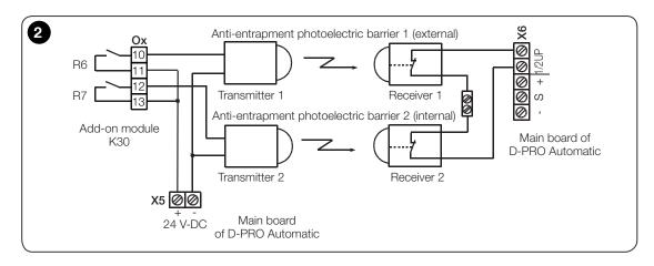
**ATTENTION**: If two photoelectric barriers are used as an anti-entrapment safeguard, the relay contacts (opening contacts) of the receivers must be switched in series and connected at terminal J33 on the main board of the D-PRO Automatic Door Control.
