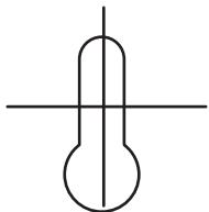
**EN** Template outline drawing of siren **MASO1** to be cut out at used to mark fixing points on the wall (to scale 1:1)
