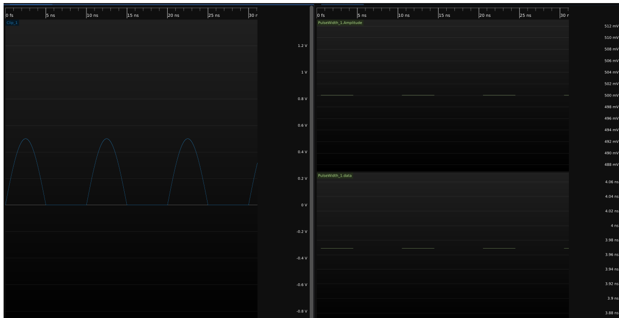
Figure 24.36: Example of pulse width measurement of a clipped sinewave input waveform.
