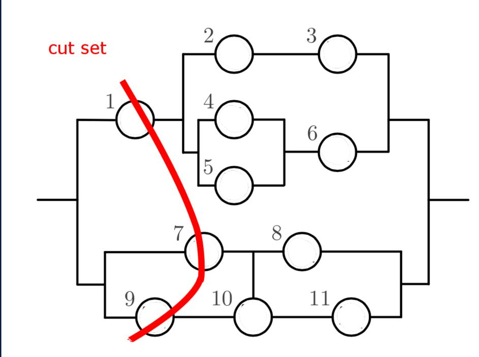
Thus, the failure time for the system depends on the system structure (via C) and the failure time distributions for each node.
