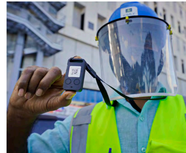
Bluetooth proximity wearables were issued to workers at JTC Logistics Hub as part of a pilot between JTC and Kimly to ensure a safe restart to operations
