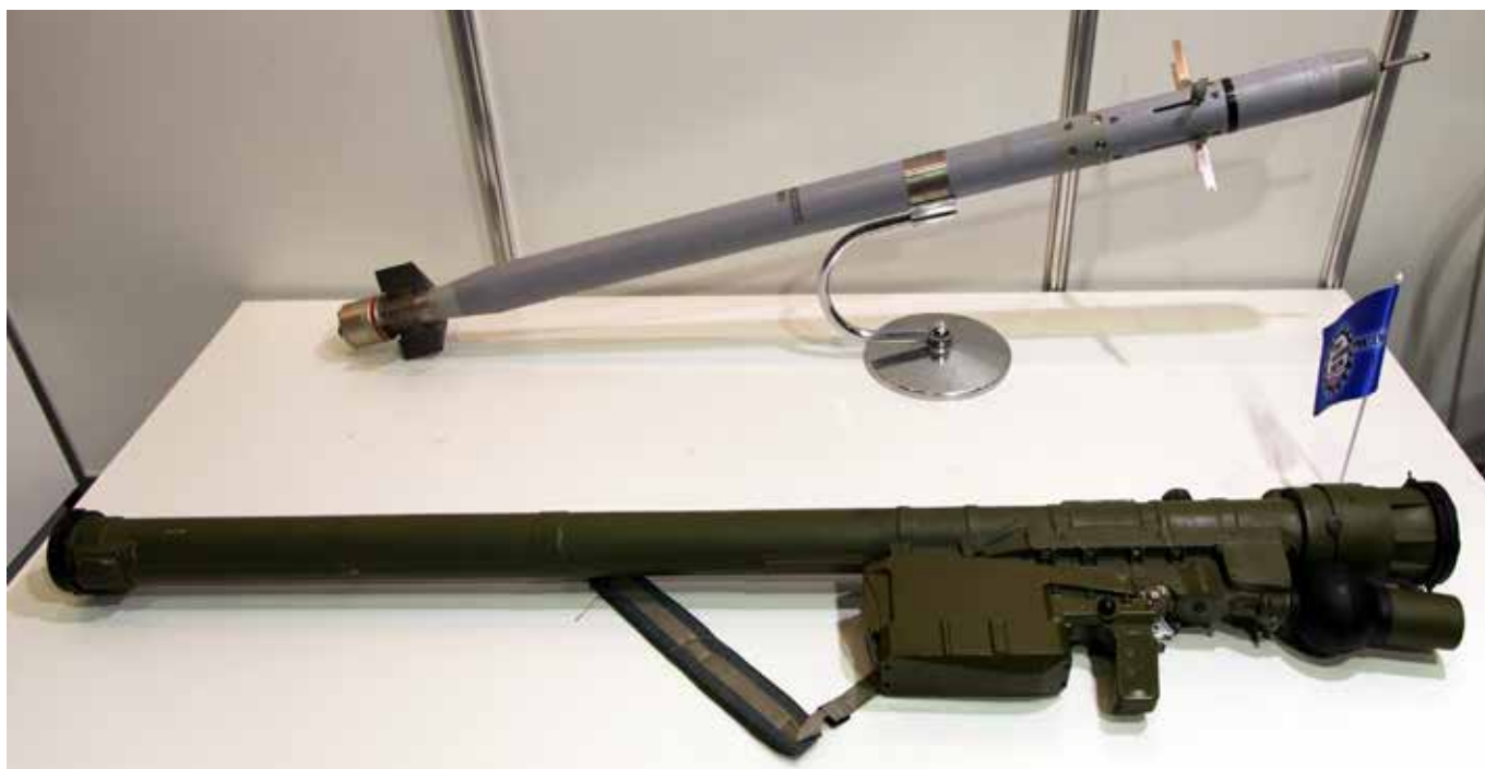
An SA-24 Iгла-S MANPADS launch tube and missile.
