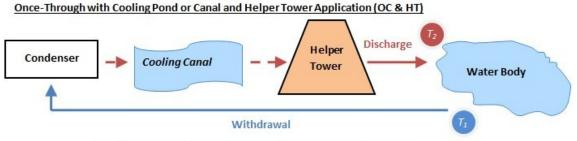
\* Helper Tower can be positioned before, after or along the canal.
