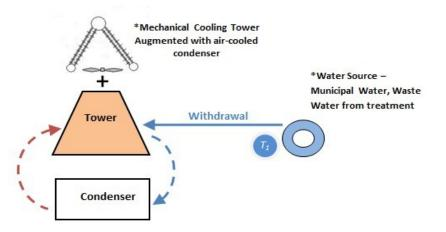
Withdrawal: Report the cooling tower makeup water that is removed from a water body.
