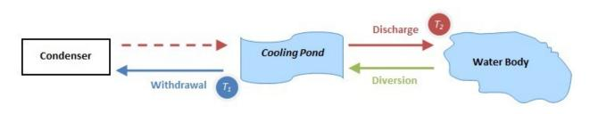
Withdrawal: Report the water flow to the condenser from the cooling pond.
