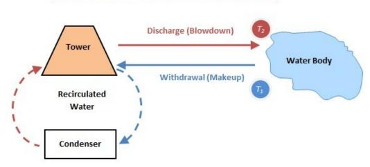
Recirculating System with Tower and No Pond (RN, RI, RF)
