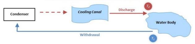
Withdrawal: Report the water that is removed from a water body for cooling, i.e. water used through the condenser.
