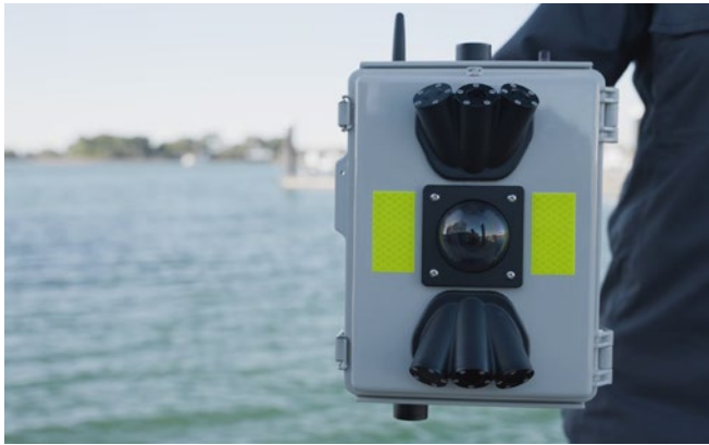
CSIRO's HydraSpectra sensor for installation at the AquaWatch pilot site at Keppel Bay on Darumbal Sea Country, monitoring sediment and dissolved carbon flow from the Fitzroy River towards the Southern Great Barrier Reef.
