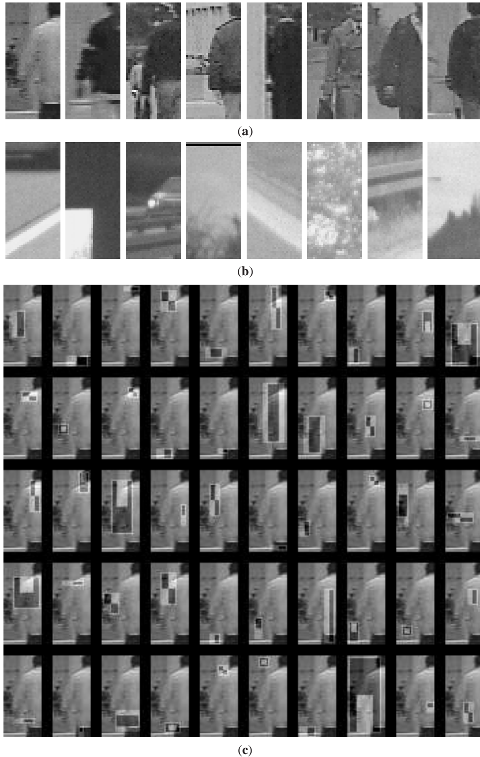
Figure 4.6: AdaBoost detector for the left side of an upper body. Typical positive and negative examples are shown in (a) and (b) respectively. All positive examples were selected in a supervised fashion and scaled to a canonical size of 28 \times 60 pixels. Negative examples were picked at random from a set of street images that did not contain people. The negative set was then refined using bootstrap procedure. The features selected by AdaBoost, overlaid on an example image of the upper body, are shown in (c). The final strong classifier learned consisted of 50 features shown in (c) weighted by corresponding \alpha_k 's (not illustrated).
