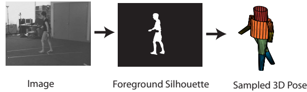
Figure 6.1: Typical discriminative inference process. Discriminative approaches [2, 3, 4, 189, 206] attempt to estimate the 3D pose directly from the image features, as illustrated above.
