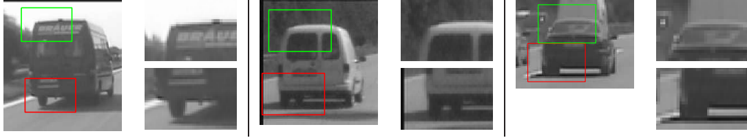
Figure 4.1: Variation within the class of vehicles. Three instances of vehicles are shown, with two different types of vans on the left and middle and a smaller passenger car on the right. While vehicles shown here have a drastically different appearance as a whole, due to the varying height and type of the vehicle, their components, illustrated by red and green rectangles, tend to be very homogeneous and are easy to model. The components, for convenience, are also illustrated separately to the right of each corresponding vehicle. Notice that components corresponding to the top-left corner of a vehicle, all have distinctive 90 degrees rotated ‘L’ shaped open contour structure; components corresponding to the lower portion of vehicles have a distinctive tire profile in all cases. The relative position of these components is, however, different in each case.
