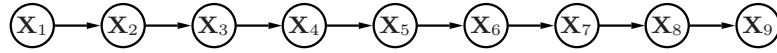
Figure 3.3: Markov Chain. Graphical model corresponding to a first-order Markov Chain. First-order Markov assumption encoded in the model presumes that the state, \mathbf{X}_t , at time t is only a function of the state at t - 1 for all t \in [2, \dots, T] , where in the example above T = 9 .
