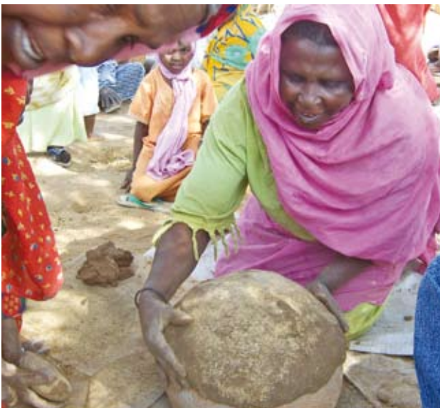
Pic 43. The mould is turned over and the clay is pressed on top of it.
