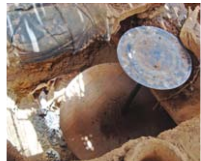
Pic 11. The potter's wheel set up in a factory (The wheel bat at the top).
