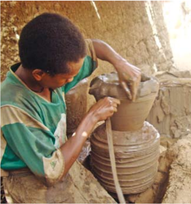
Pic 32. Further clay is added and tape is wrapped around the fatela 1 and the new material. This happens at each stage.
