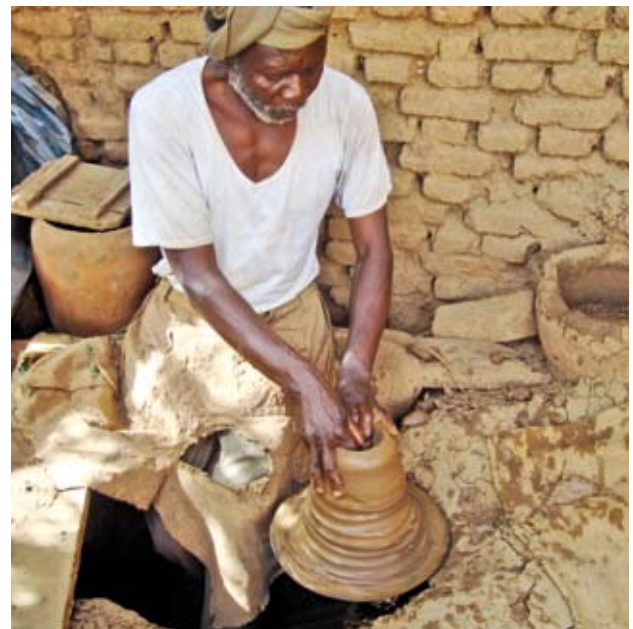
Pic 24. The potter finds the center of the clay by moving a thumb across the lump until no more friction is felt. The fingers are pressed into the center of the lump to form a hole.
