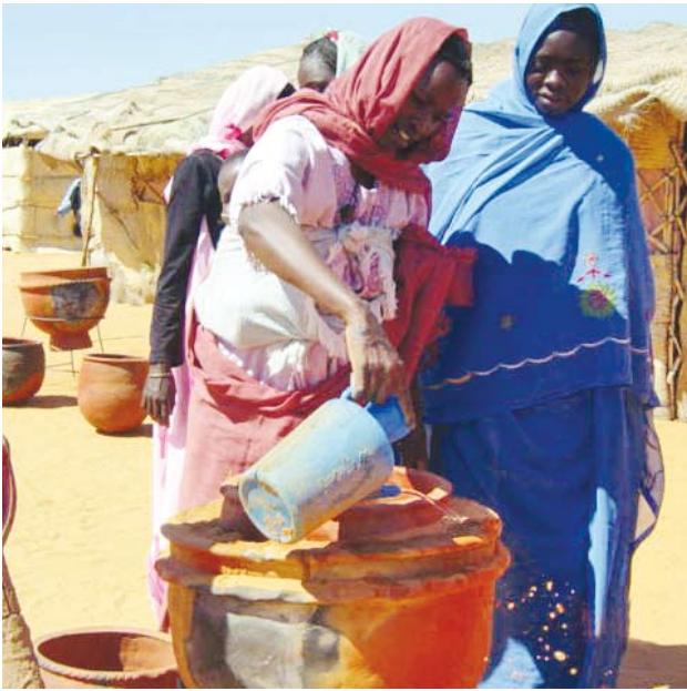
Pic 48. When the refrigerator is assembled water is poured on the sand.
