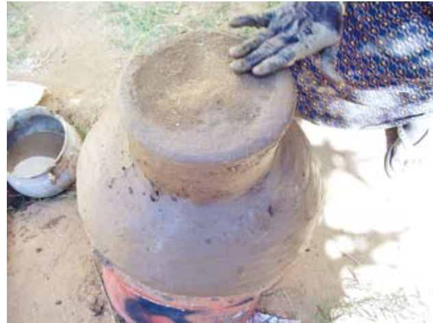
Pic 69. The base is secured and blended in with the rest of the stove.
