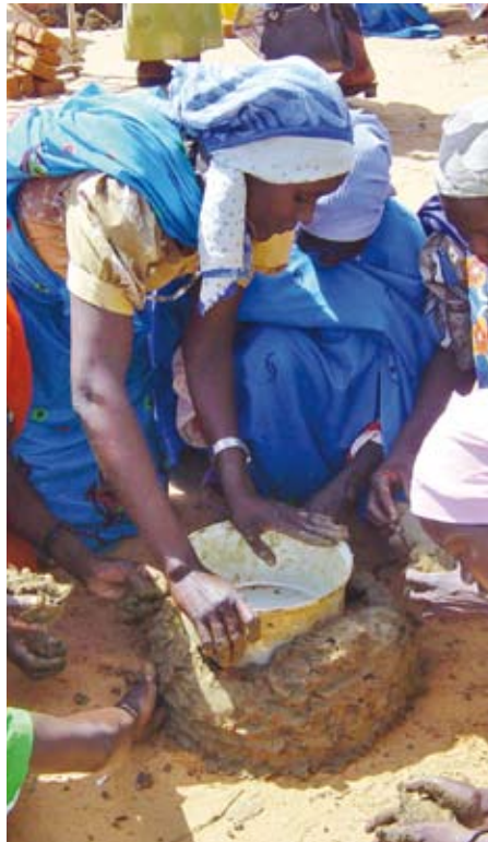
Pic 9. Ladies using the saucepan as a mould for the improved clay stove.
