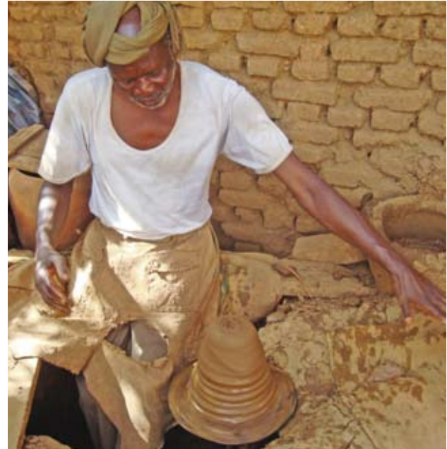
Pic 23. The potter throws the clay on the spinning wheel bat. The lump is made even and forced to the centre of the wheel by applying pressure with the hands.
