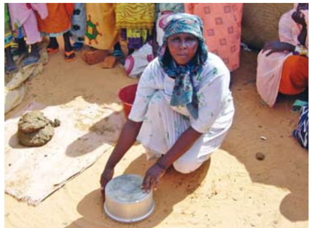
Pic 54. A line is drawn around the outside of the saucepan most frequently used in the kitchen to determine the size of the stove.
