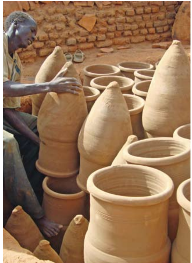
Pic 38. The zeers are assembled in the kiln ready for burning. The kiln fuel is wood which is lit under the zeers, see picture 39 for kiln.
