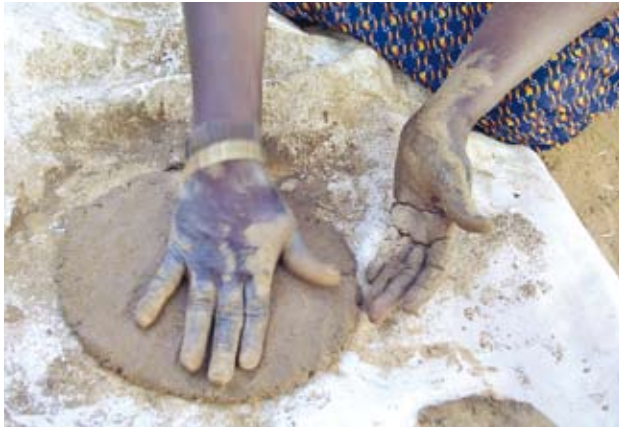
Pic 67. A flat circle of clay is formed which will be the base of the stove.
