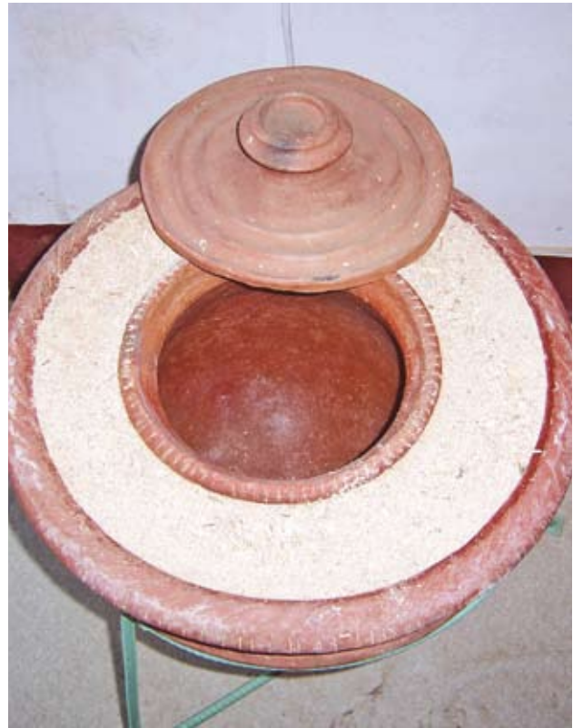
Pic 49. An assembled refrigerator using wood chippings for insulation.
