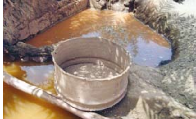
Pic 19. The filter bucket has lots of little holes in the bottom for drainage.
