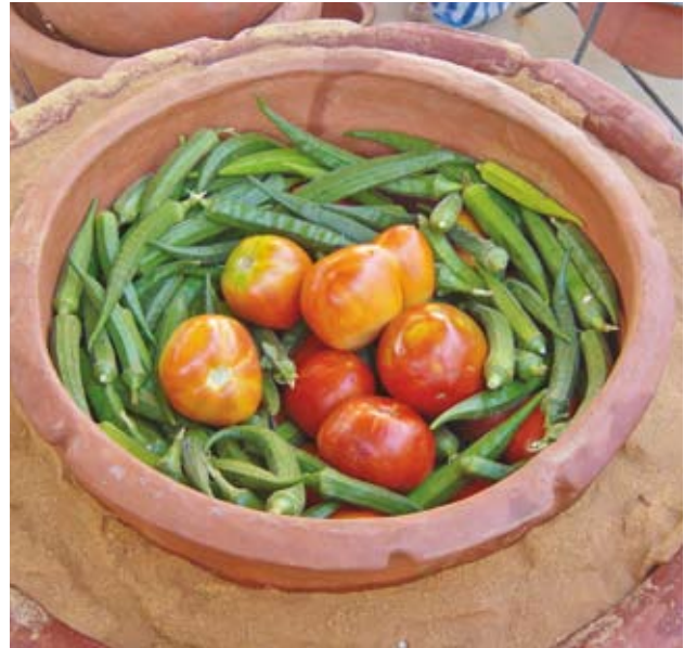
Pic 50. An assembled refrigerator using sand for insulation.
