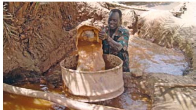
Pic 20. The mixture is transferred by hand through the filter to get rid of the impurities into the filtered hole.
