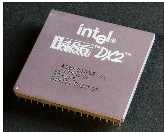
Intel 80486DX2 top , Intel 80486DX CPU. Top view with screen printed logo and component ID markings. ---- Photograph © Andrew Dunn, 9 November 2005, CC BY-SA 2.0
