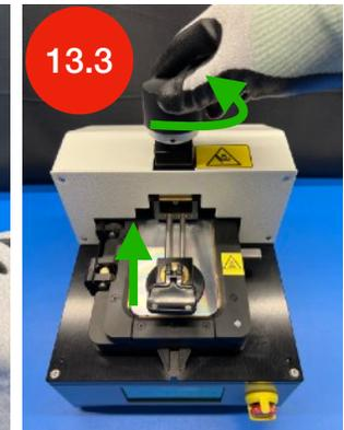
14. The phone display is now separated. Disengage the suction cup from the top of the display to release the suction cup from the display
