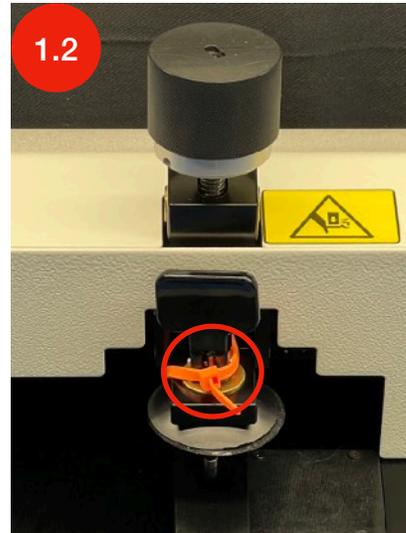
2. Move the suction cup arm to the highest position by rotating the torque limit handle counter clockwise
