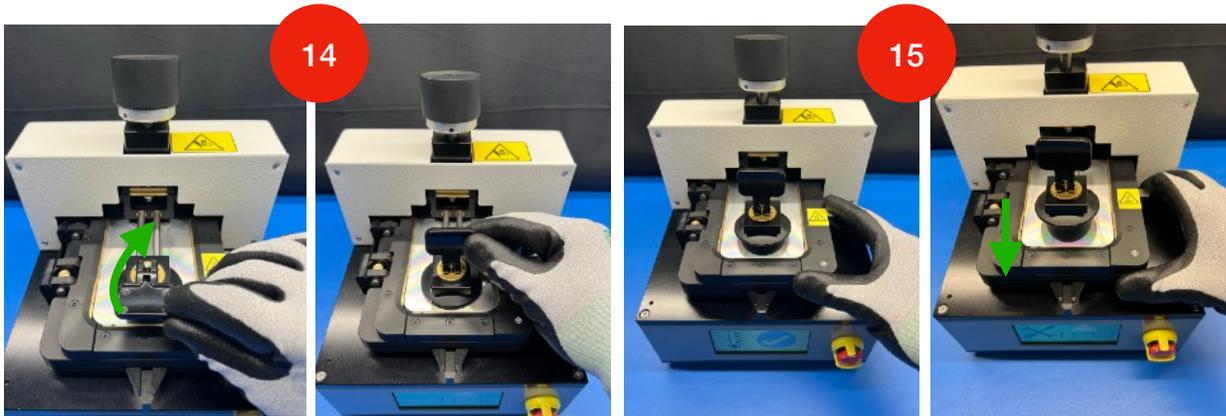
16. The display has now been separated and the fixture is now back to STANDBY MODE (Yellow LCD) and ready for another use cycle
