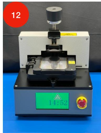
13. The fixture is now in OPEN MODE (Green LCD) - and a Countdown Timer of 15:00 minutes will appear, the technician has 15:00 minutes to complete the separation of the assembly. If the separation is not completed and the nest is not ejected in 15:00 or less, the power to the nest will turn off automatically.
