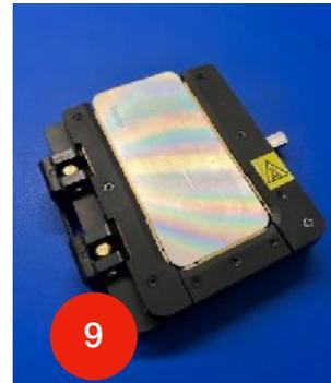
10. Insert the nest with the phone into the fixture
