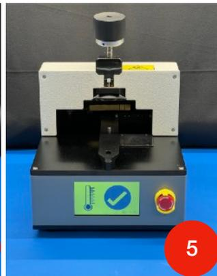
6. Ensure that the Heated Display Pocket is in the 'Open' position with toggle levers flipped up
