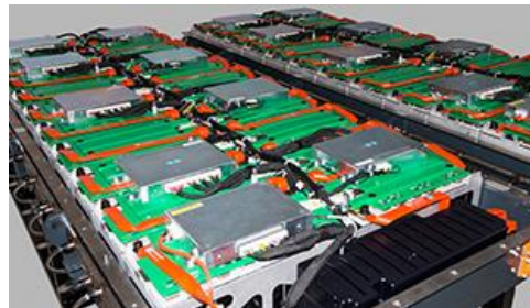
Battery management system
