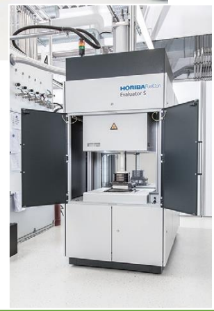
Right: Battery, fuel cell, electrolyzer evaluation device "Evaluator"
