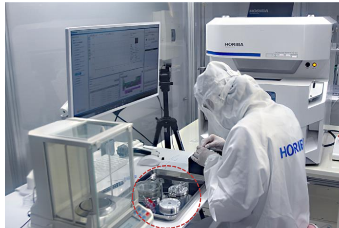
Analyzing the sample with our X-ray fluorescence
