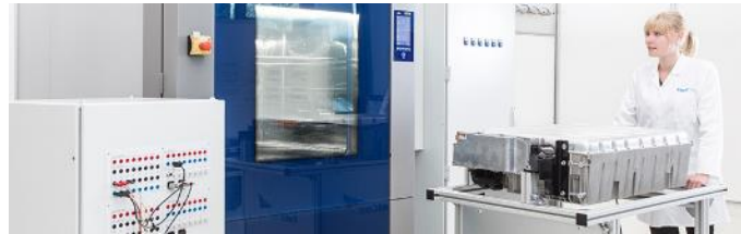
Battery module/pack test system
