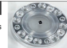
Developed a special container (cell) to allow advanced handling of sample materials from Ryugu
