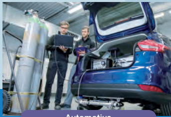
Emission measurement; engine development Contributes to engine development and meeting emission regulations
