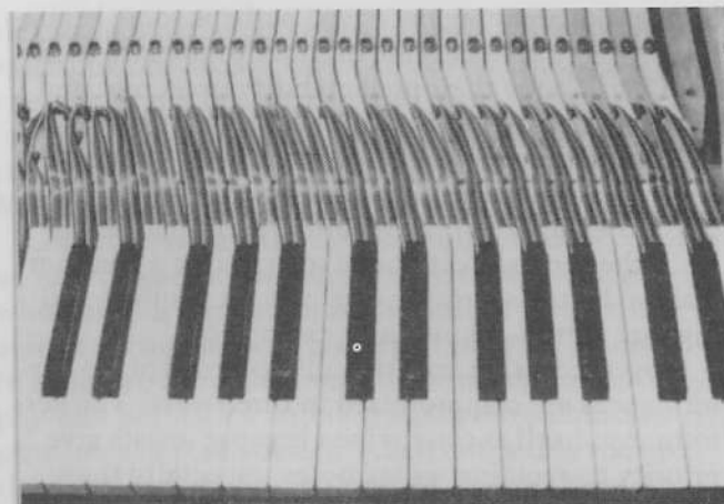
Fig. 5. A portion of a Yamaha CP-80 Piano keyboard, showing the XY key surface sensors. Note that white key surfaces are coated with white epoxy in this example.
