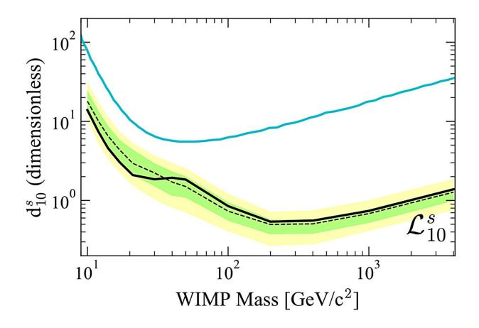
The limit on the couple strength of a WIMP-nucleon interaction as a function of WIMP mass at the 90% confidence limit (black line). Results from PandaX-II (blue) are shown for reference. We can think of "d" as the strength of this particular interaction type. Credit: LZ Collaboration
