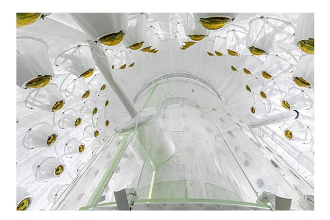
The LZ detector is a set of three nested detectors meant to sense the smallest amounts of energy deposited by radioactive materials or dark matter. Seen here is the LZ Outer Detector that encloses the skin veto, and the 10 tons of liquid xenon in the LZ TPC. Credit: LZ Collaboration.
