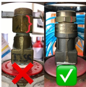
Figure 32: Older vs. newer spindle design. Strongly advise all to only accept cylinders with newer spindle design.
