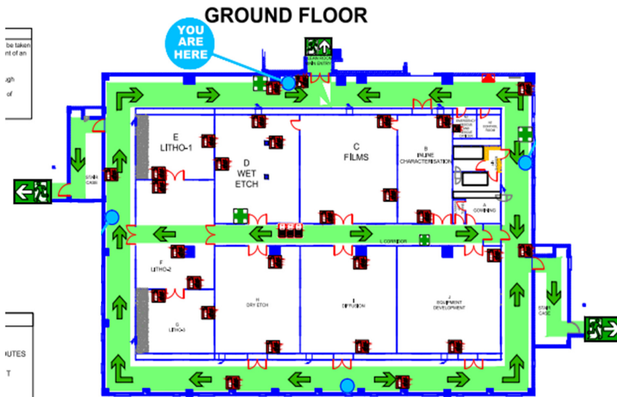
Figure 35: Example of an emergency escape route
