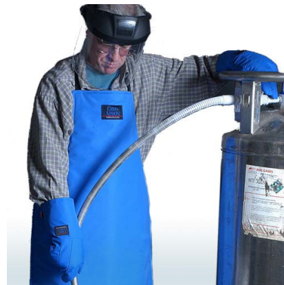
Figure 28: The correct usage with proper protective equipment + use of both hands to hold the tank and tube.
