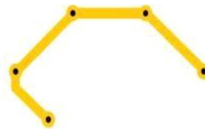
Connection via continuous trace
