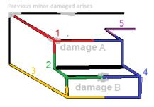
Each damage can be just one time measured on arises as shown in the pictures by the samples damage A (corner) or damage B (arise).
