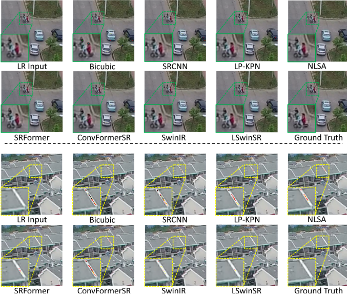
Fig. 2. Visual comparison of SR ( \times 2 ) images between different methods on training (top) and validation (bottom) sets for segmentation.
