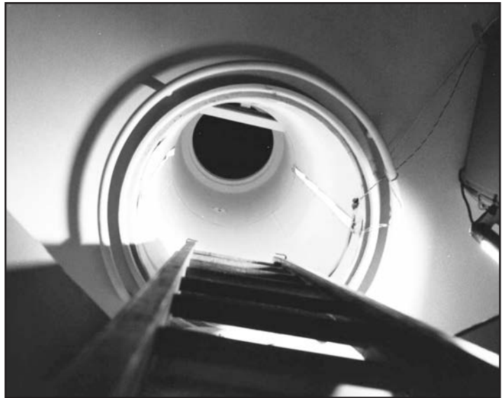
Tunnel connecting the laboratory module and Gemini capsule. Source: CSNR Reference Collection.
