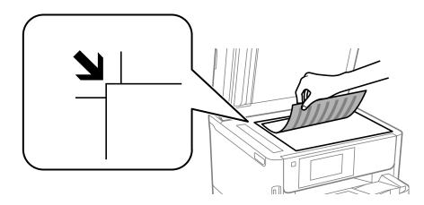
**Note:** The edges of your original may be cropped by 0.06 inch (1.5 mm) from the edge of the scanner glass. Manually position your original away from the edges to prevent cropping.
