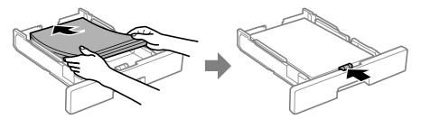
Note: Make sure the paper fits beneath the arrow mark inside the edge guides.
