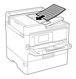
**Note:** Do not load originals above the arrow mark on the ADF edge guide.
