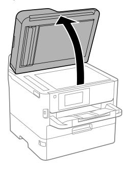
2. Place your original facedown on the scanner glass with the top facing into the corner. Slide the original to the edges of the indicated corner.
