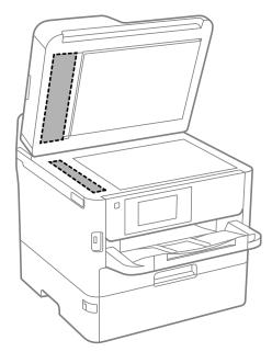
**Note:** If lines appear on the printout or in scanned images, carefully clean the scanner glass on the left.
