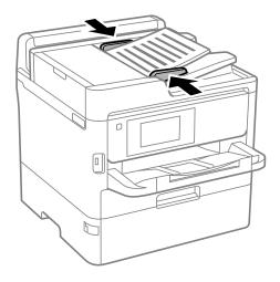
**Note:** If you are copying two originals onto one sheet, make sure the originals are loaded as shown. Select the link below to select the copy orientation setting that matches how you loaded your original.
