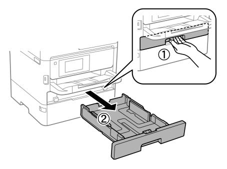
Note: If the optional paper cassette unit is installed, do not remove more than one cassette at a time.
