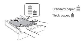
**Note:** Make sure the paper is under the arrow mark for your paper type and loaded against the front edge of the cassette.
