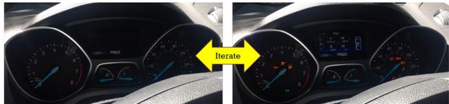
(b) Adversaries can inject messages into the CAN bus of the vehicle to prevent the system from falling asleep [93].
