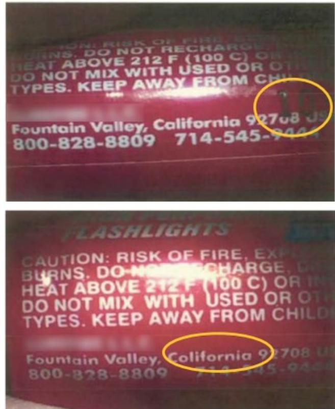
Fig. 7. An authentic battery (top) v.s. a counterfeit one (bottom). Counterfeit one has a misspelled 'California' and a missing stamp [51].
