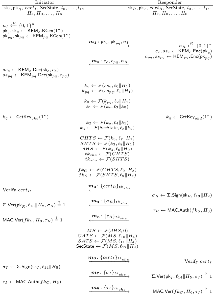
Fig. 2. One stage of the Muckle+ protocol with a classical KEM \text{KEM}_c , a post-quantum KEM \text{KEM}_{pq} , a MAC \Sigma , and a PRF \mathcal{F} whereas k_q represents the symmetric key from the QKD component (provided out-of-band via function \text{GetKey}_{qkd} ). cert_I and cert_R are certificates (provided out-of-band) for the public keys pk_I and pk_R , respectively. CATS and SATS are the client and server application traffic secrets, respectively. Messages m_i: \{m_{i,1}, \dots\}_k denote that m_{i,1}, \dots is encrypted with an authenticated encryption scheme using the secret key k . The various contexts and labels are given in Tables 2 and 3.
