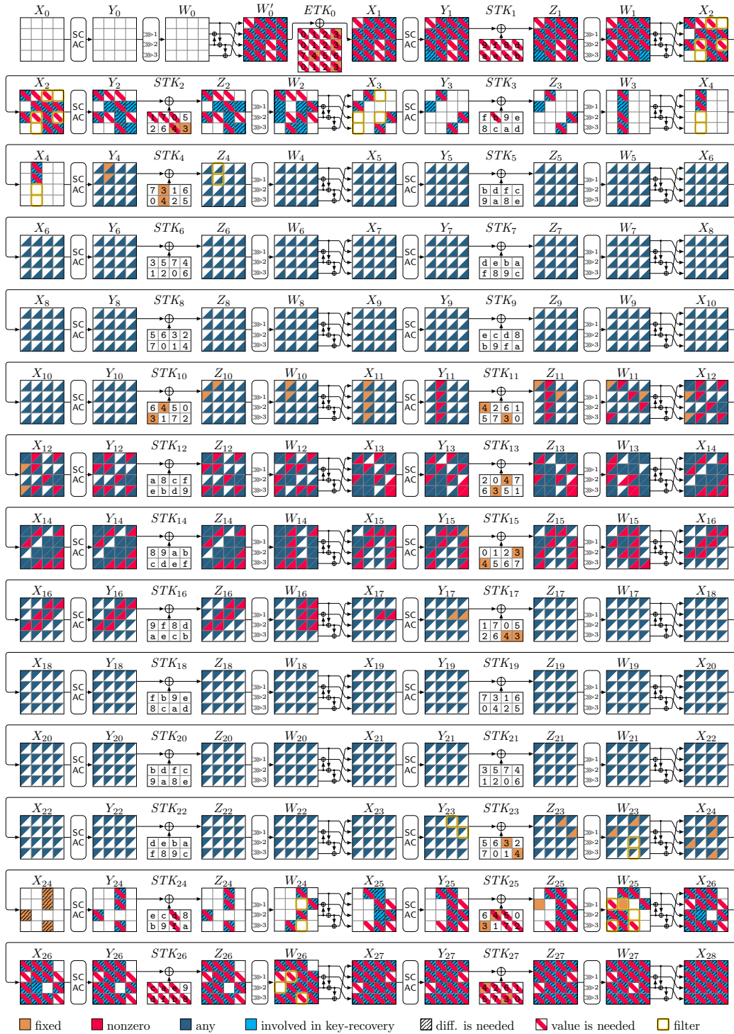
Figure 29: Related-Tweakey ID attack on 28 rounds of ForkSKINNY-64-192-192 in the limited setting ( r_i = 11, r_0 = 17 ). |k_B \cup k_F| = 160 , c'_B = 52 ( c_B = 44 ), c_F = 56 , \Delta_B = 52 , \Delta_F = 56 . In this case we have 15 \times 15 related-key impossible differences.
