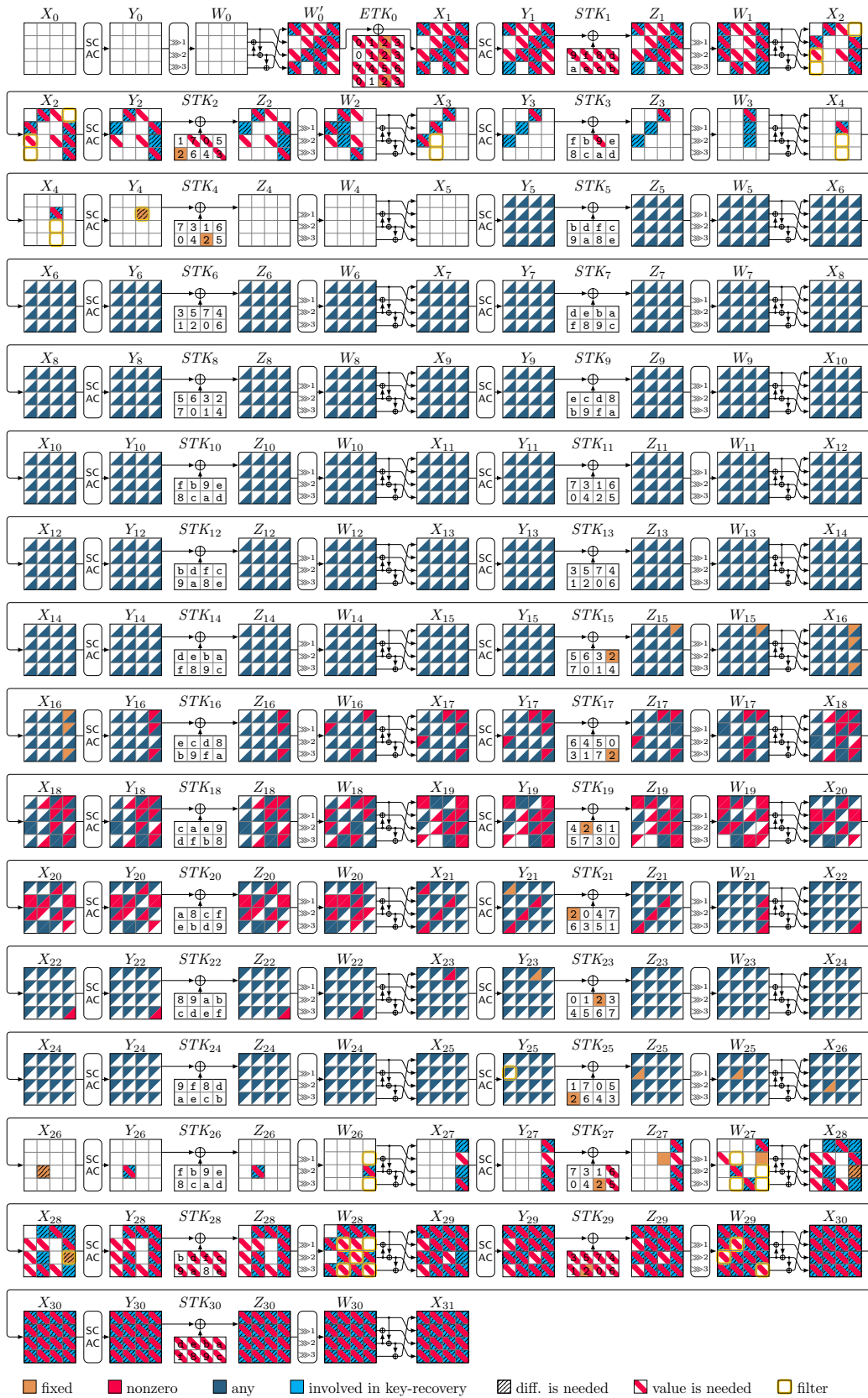
Figure 37: Related-Tweakey ID attack on 31 rounds of ForkSKINNY-128-288-288 in the arbitrary setting ( \mathbf{r}_1 = 10, \mathbf{r}_0 = 25 ). |k_B \cup k_F| = 272 , c'_B = 64 ( c_B = 56 ), c_F = 128 , \Delta_B = 64 , \Delta_F = 128 . In this case we have 15 related-key impossible differences.
