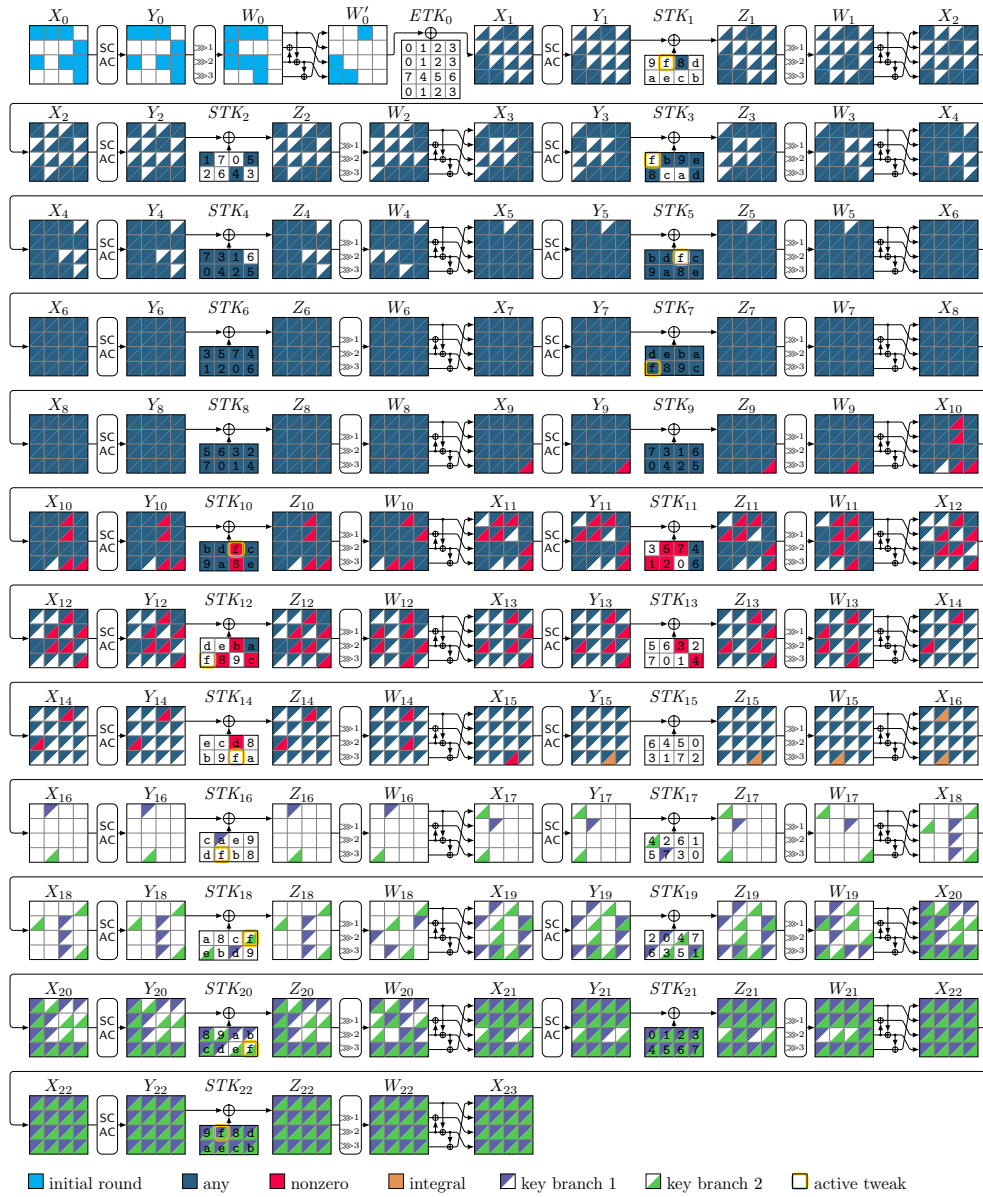
Figure 19: ZC-based integral attack on 23 rounds of ForkSKINNY-128-256.
