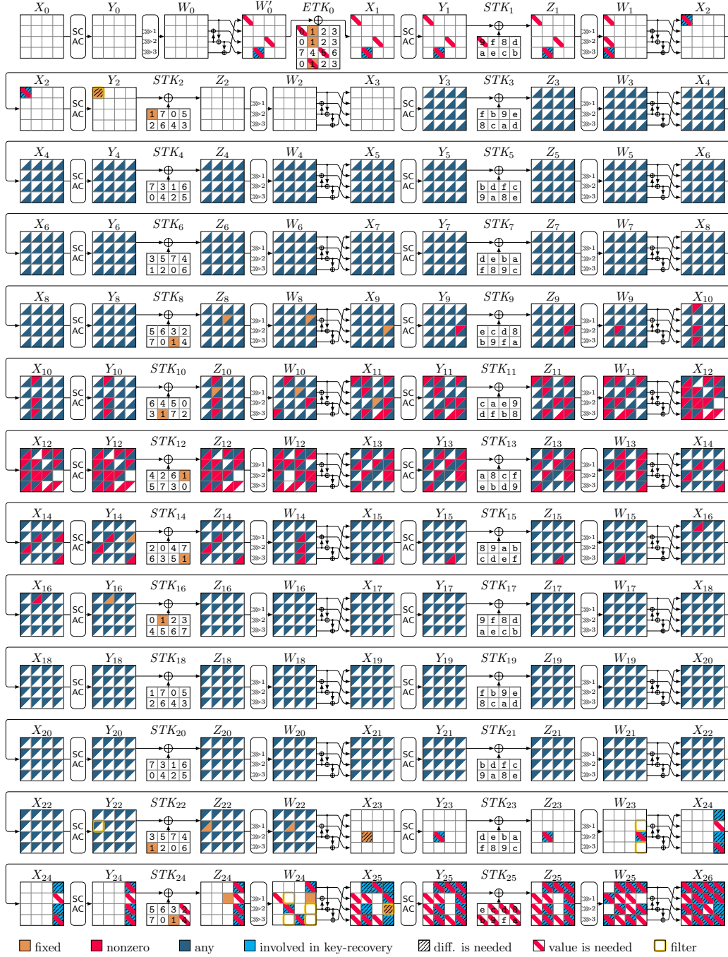
Figure 40: Related-Tweakey ID attack on 26 rounds of ForkSKINNY-128-288-128 in the limited setting ( r_i = 10, r_0 = 16 ). |k_B \cup k_F| = 88 , c'_B = 8(c_B = 0) , c_F = 64 , \Delta_B = 8 , \Delta_F = 64 . In this case we have 15 related-key impossible differences.
