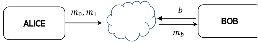
Figure 1. Oblivious Transfer begins with Alice (the sender) posting two messages m_0 and m_1 . Bob (the receiver) privately and randomly selects a bit b and recovers the corresponding message m_b , but nothing more. Alice does not acknowledge the selected bit from Bob and Bob ignores the unselected message.
