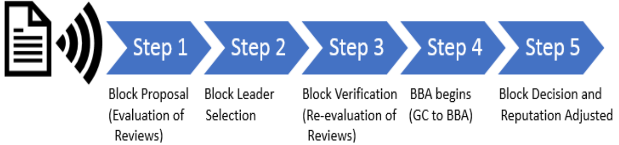
Figure 5: The five steps simplified for discussion on the Proof of Review extension. There are other virtual steps that form a cycle from these last steps to ensure convergence but are omitted since it is not directly relevant in respect to our review system. If interested, see [1]
