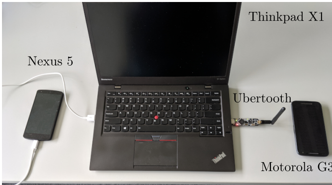
Fig. 7: Our evaluation setup. In the Bluetooth case, we use a Nexus 5 both as a victim and the attacker, a Motorola G3 as a victim, and a Thinkpad X1 laptop to patch the Nexus 5’s Bluetooth firmware. In the BLE case, we use a Thinkpad X1 both as the attacker and as a victim. The laptop runs our custom Linux kernel and user space stack. In both cases, we eavesdrop the packets using an Ubertooth One.
