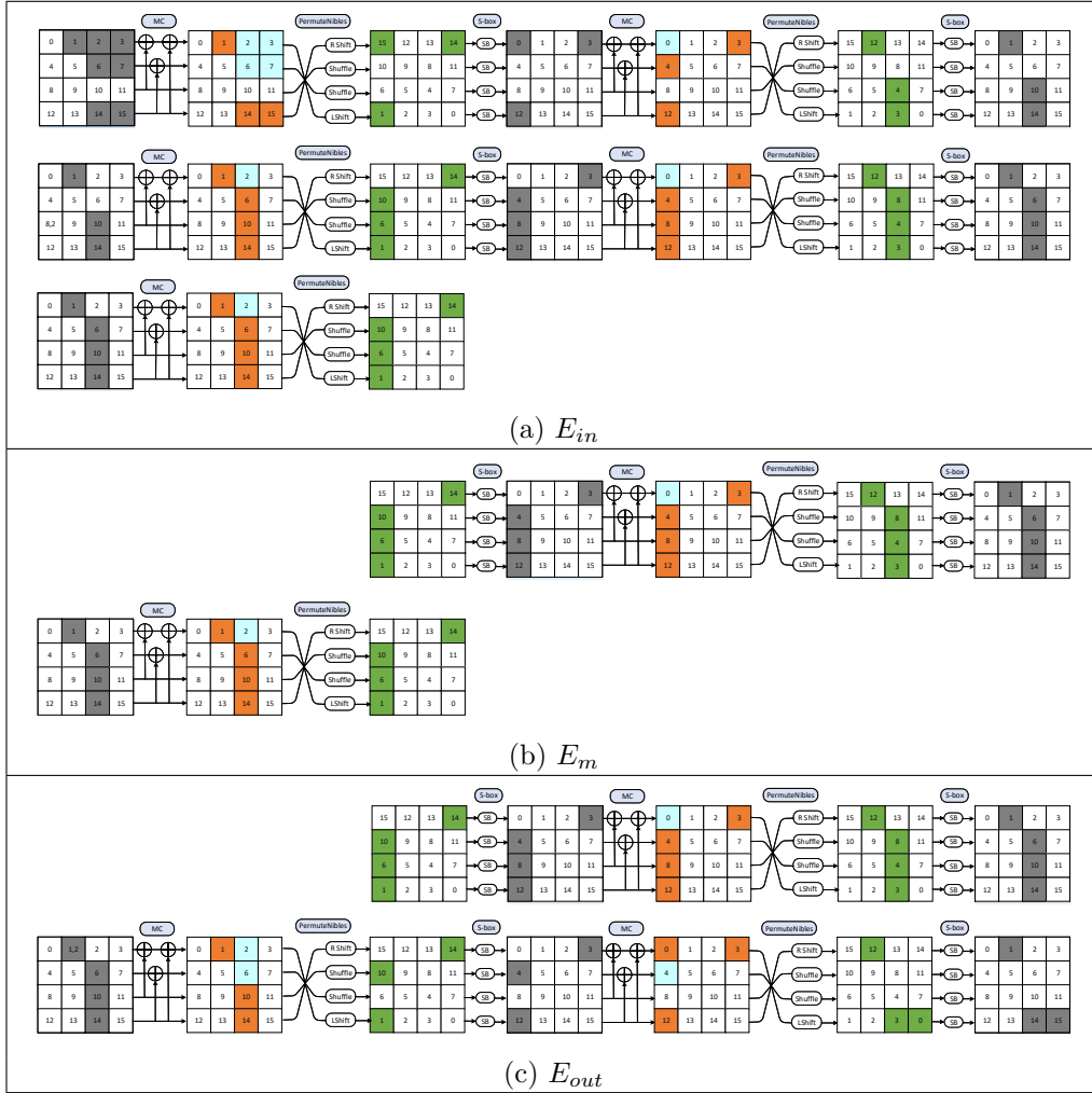
Figure 4: An expendable truncated trail for even rounds, where E_{in} and E_{out} denote the first 4 and the last 4 rounds, respectively and E_m is a repeatable 2-round truncated trail that can be used as much as required. For example, to design a 10-round trail, this stage is repeated once in the current trail. The Cyan-colored cells are inactive due to cancellation after MC step, white-colored cells are inactive, and {Gray, Orange, Green} colors are active cells in different stages of the cipher.
