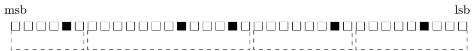
Fig. 1: Partition of a sparse integer into intervals. The blocks represent the binary expansion, the black blocks as ones and the white blocks as zeros. Interpreting an interval as integer yields a small number, e.g., the first interval represents 2^3 = 8 .
