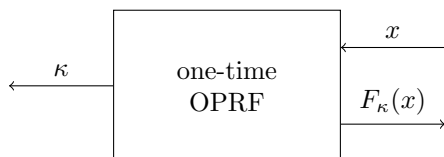
Figure 4: The one-time OPRF functionality. In the one-time OPRF functionality, the PRF key is not specified by the sender, but instead is generated by the protocol itself.
