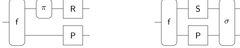
Figure 3: The real (left) and the ideal (right) setting considered in context-restricted indistinguishability for a specific context (f, P) consisting of the filter f and the auxiliary parallel resource P .
