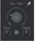
Here is the mixer for Dry & Wet. It operates like a crossfader. This control works directly with the FX Level parameter beneath it to set the balance of your mix. This parameter can be switched between **Dry/Wet** and **Dry Level** mode in the Settings menu. Dry/Wet has three dynamic/VCA trigger modes.
