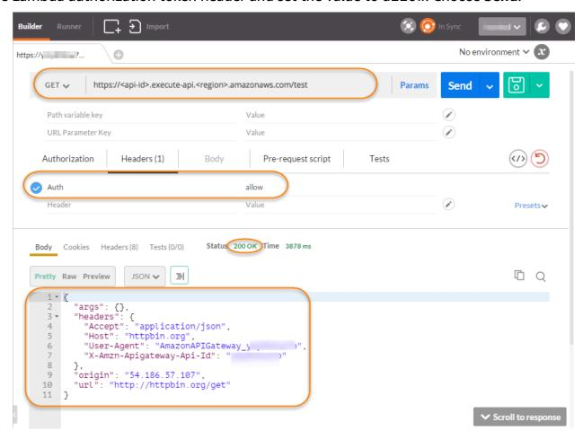
The response shows that the API Gateway Lambda authorizer returns a **200 OK** response and successfully authorizes the call to access the HTTP endpoint (http://httpbin.org/get) integrated with the method.
