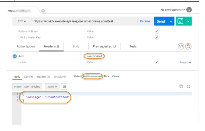
The response shows that API Gateway returns a **401 Unauthorized** response without authorizing the call to access the HTTP endpoint.
