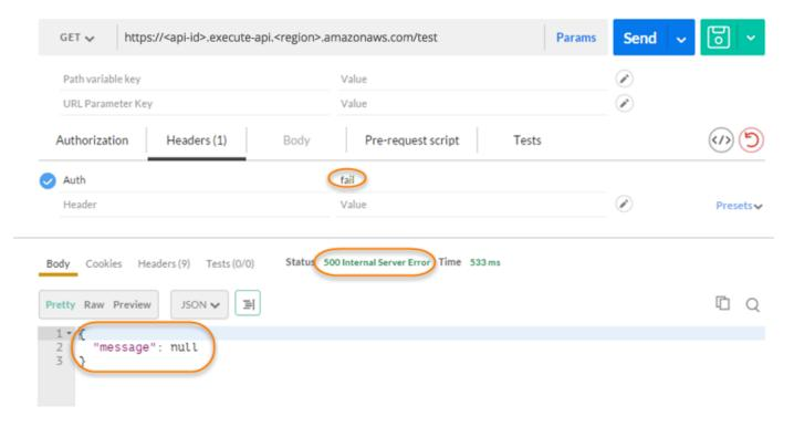
The response shows that API Gateway returns a **500 Internal Server Error** response without authorizing the call to access the HTTP endpoint.
