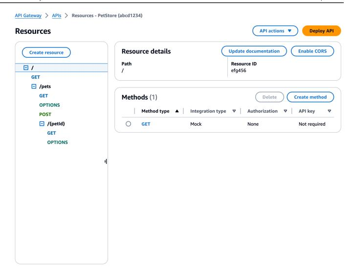
The **Resources** pane shows the structure of the created API as a tree of nodes. API methods defined on each resource are edges of the tree. When a resource is selected, all of its methods are listed in the **Methods** table on the right. Displayed with each method is the method type, integration type, authorization type, and API key requirement.
