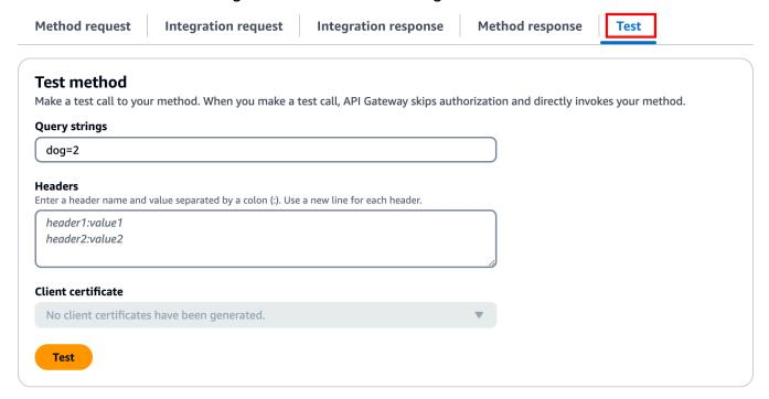
Enter values in any of the displayed boxes (such as Query strings, Headers, and Request body). The console includes these values in the method request in default application/json form.
