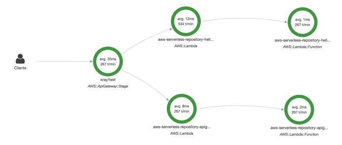
From the service map, you can zoom in to see a trace view of your API stage. The trace will display in-depth information regarding your API, represented as segments and subsegments. For example, the trace for the service map shown above would include segments for the Lambda service and Lambda function. For more information, see AWS Lambda and AWS X-Ray.
