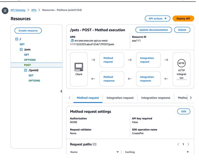
The resulting **Method execution** pane presents a logical view of the chosen (POST /pets) method's structure and behaviors.
