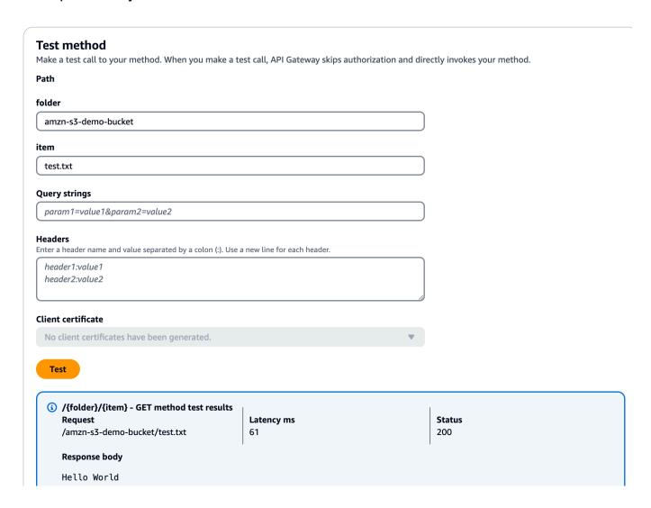
The request correctly returns the plain text of ("Hello world") as the content of the specified file (test.txt) in the given Amazon S3 bucket (amzn-s3-demo-bucket).
