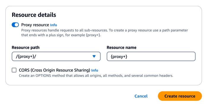
In this step, you integrate the ANY method with a backend HTTP endpoint, using a proxy integration. In a proxy integration, API Gateway passes the client-submitted method request to the backend with no intervention from API Gateway.
