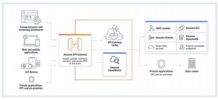
This diagram illustrates how the APIs you build in Amazon API Gateway provide you or your developer customers with an integrated and consistent developer experience for building AWS serverless applications. API Gateway handles all the tasks involved in accepting and processing up to hundreds of thousands of concurrent API calls. These tasks include traffic management, authorization and access control, monitoring, and API version management.
