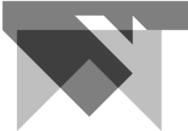
Figure 1: Two input polygons. The area shared by the polygons is shaded with the darkest grey.
