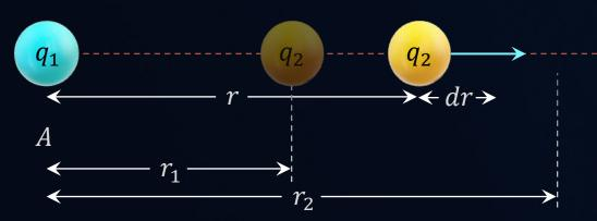
Work done by electric force in moving the charge  $q_2$  from  $r=r_1$  to  $r=r_2$ :
