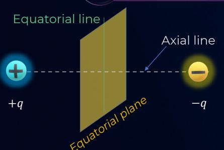
An electric dipole is a system consisting of two point charges, equal in magnitude but opposite in nature, and separated by a small distance.
