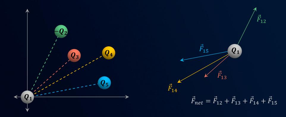
The net electrostatic force acting on a given charge is equal to the vector sum of electrostatic forces exerted on it by all the other charges in its surroundings.
