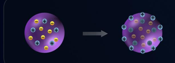
• Excess charge given to an isolated conductor redistributes itself on the surface in order to minimize the potential energy/maximize stability.
