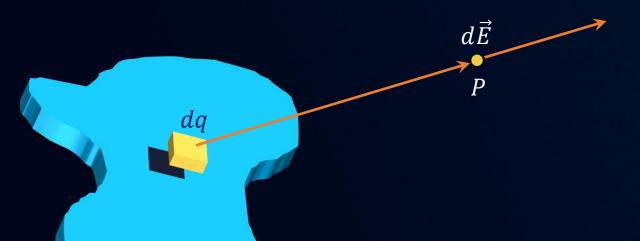
Electric field at point P due to an infinitesimally small, charged element dq of the continuous charged body is,
