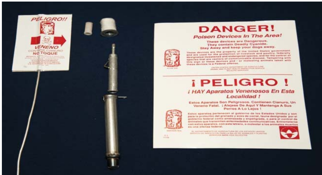
The M-44 ejector device consists of a capsule holder, a small plastic container holding sodium cyanide, a spring-activated ejector, and a stake. Bilingual warning signs are required to mark their placement.
