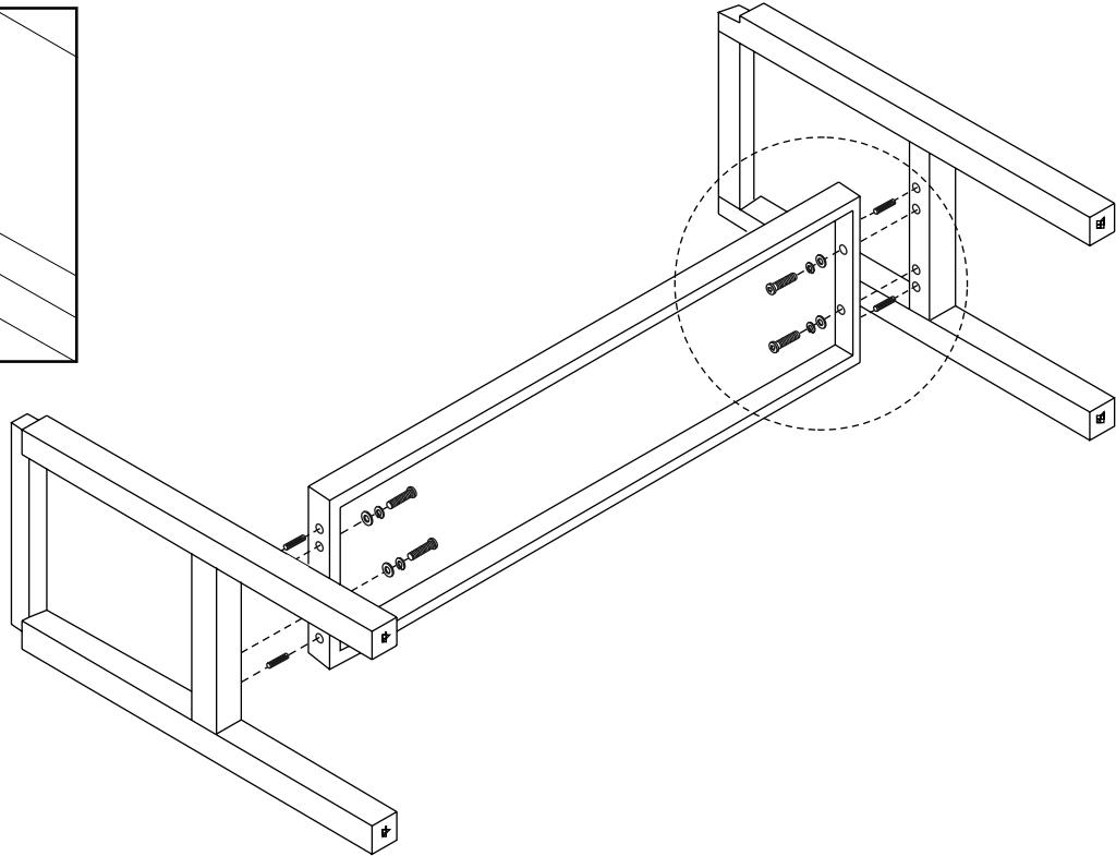
2. Align top and base as shown. Insert bolt (A), lock washer (C), and flat washer (B). Tighten with supplied hex key (E). With help stand bookcase upright.
