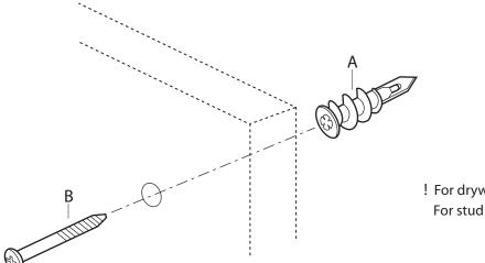
! For drywall mounting, use anchors with screws. For stud mounting, use screws only.
