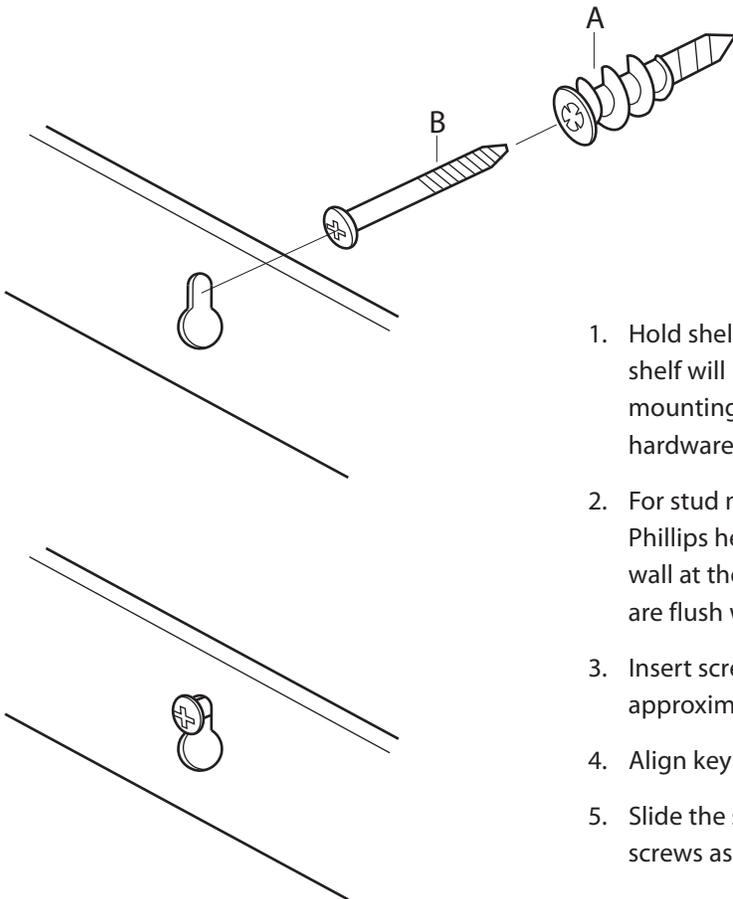
! For drywall mounting, use anchors with screws.
