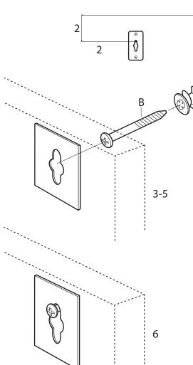
! For drywall mounting, use anchors with screws. For stud mounting, use screws only.
