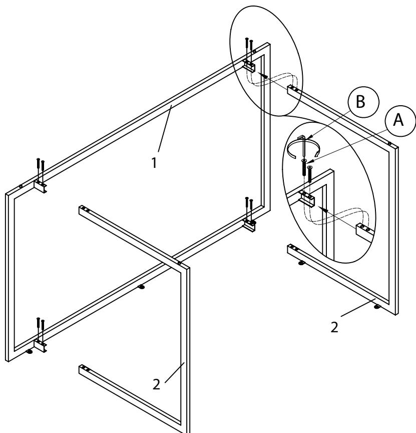
2. Lay the top (part 3) upside down onto a clean smooth surface such as carpet or cardboard. Align the assembled parts from step #1. Insert bolt (A) and tighten with supplied hex key.
