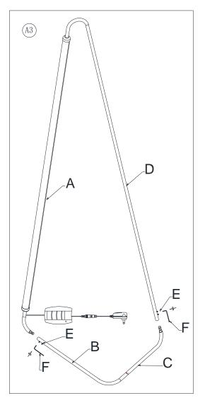
3. Turn the assembled Tubes (A&D) upright and hold by another person. Connect the bottom tube assembly (B&C) with the standing tube assembly (A&D) like shown and secure with the 4 Set Screws (E). Make sure that all parts are connected in right position. Now fully-tighten all 8 Set Screws (E) with the Allen Wrench (F).
