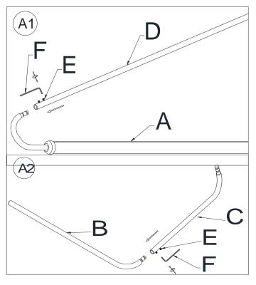
Lay the parts on a clear, flat surface as shown. Insert the Supporting Tube (D) onto the upper connection head of Lighting Tube (A) and secure with the 2 Set Screws (E). Do not fully-tighten these Set Screws (E) provisionally.
