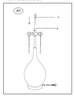
Screw the Shade Holder Pipe (C) into the Cluster Body (D)
