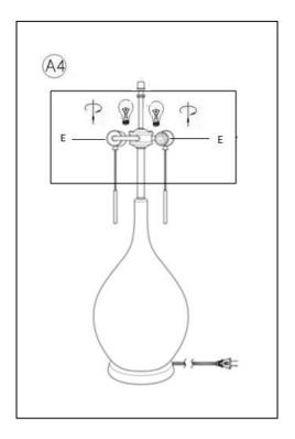
Insert the specified light bulbs into the Sockets (E). DO NOT EXCEED THE SPECIFIED WATTAGE.
